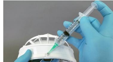
2. Dispense enough Gorilla Glue into the Front adapter to completely cover the Snap Stud.
