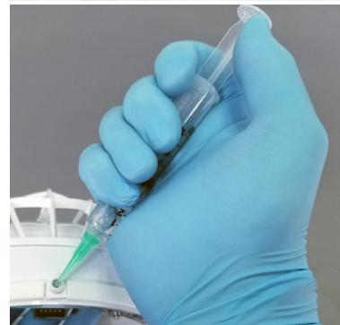
3. Draw off (siphon back into the Syringe) any excess glue. The glue only needs to completely cover the silver colored metal Snap Stud.
